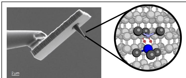
**Figure 1** – The NV center is a point defect which acts like an isolated atomic system “caged” by the diamond lattice, allowing us to observe the interesting quantum behavior of atomic systems in a solid-state platform. The samples in this workshop are diamonds which have been fabricated into cantilevers (left) with a single NV center at the pillar apex. In all the measurements, we’ll be probing the dynamics of a *single spin*.
